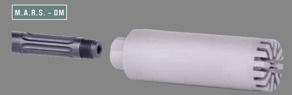
The M.A.R.S. - DM (directly mounted) is the lightest and shortest assault rifle suppressor B&T currently produces. It is screwed directly on the barrel of the weapon. This lack of any mounting system allows it to be almost 300 grams lighter and 50 mm shorter than other suppressors with a mounting system. Therefore the impact on the balance of the weapon and the extension of the gun is negligible and not perceptible in combat.
